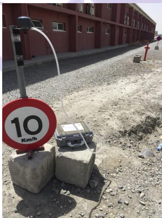
Image 4. Portable monitoring equipment set up by Preventative Medicine teams to collect particulate matter on to a filter. This filter is sent to the US for analysis. Note the clear weather that is not truly representative of a typical polluted day in Kabul.
