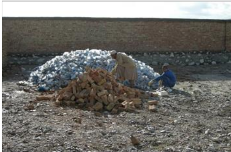
Image 2. Solid waste transported from NATO bases is sorted at the contractors yard. All valuable components of solid waste are extracted and either reused or recycled.
